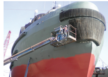
A zinc primer can be used in a variety of applications, saving time and money by eliminating the need for an intermediate coat.
