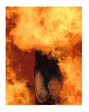
Thermo-Lag E100 saves lives and assets. When exposed to a fire it intumesces or swells, producing a heat blocking char which insulates the steel from exposure to high temperatures. This allows more time for people to exit and firefighters to respond.
